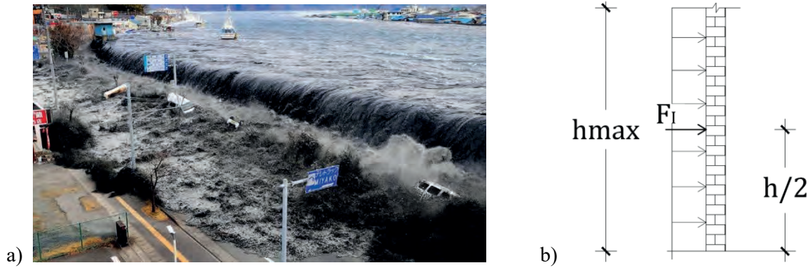
Figure 17. (a) Impact of tsunami (Tohoku 2011, Japan) , (b) Impulsive force acting on the centroid of the masonry infill
