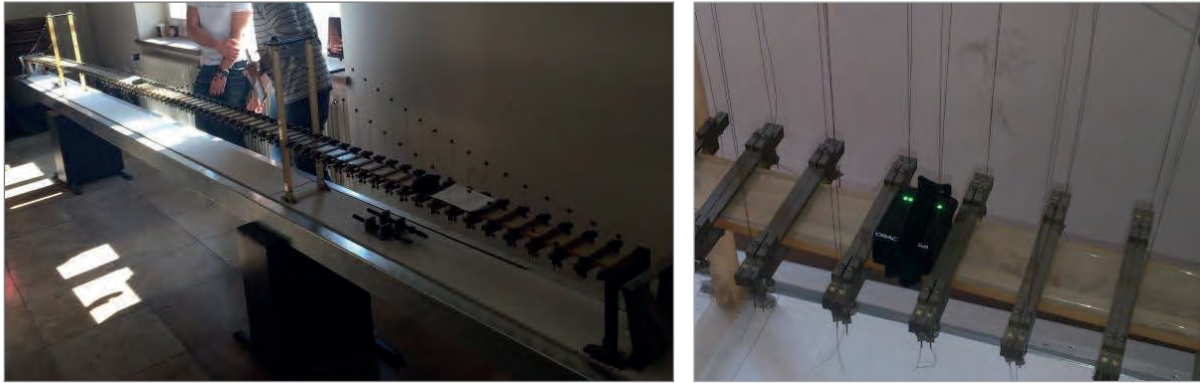
Figure 3. (a) Laboratory model of the New Little Belt suspension bridge (scale of 1:200) and (b) a mounted SunSPOT node
